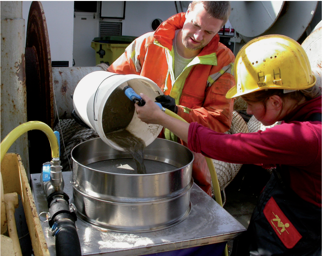
Figure 16 Samples of the macrobenthos are collected by means of a Van Veen grab and passed over a sieve with a mesh size of 1 mm.
