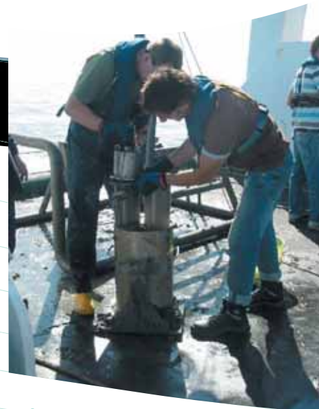
Taking samples to determine the sediment erodibility
