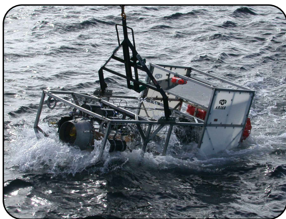
Towed sampling equipment developed by FRS for surveying Calanus in the deep ocean during their winter hibernation phase.
