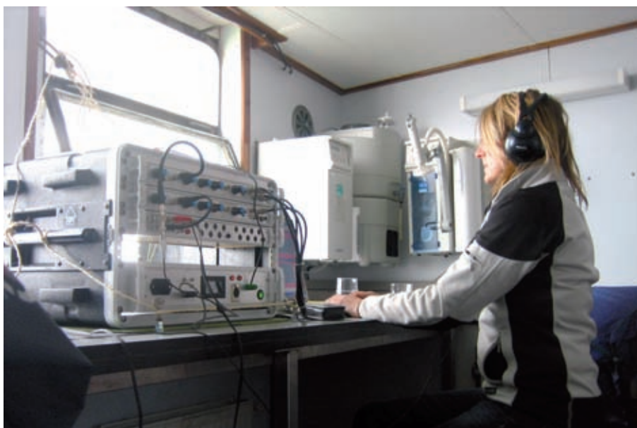
Within the framework of the systematic bird and marine mammal counts of the Research Institute for Nature and Forest (INBO) VLIZ takes care of the purchase, management and operation of a Passive Acoustic Monitoring (PAM) system. These hydrophones are an additional source of information on the occurrence of porpoises and other delphinoids in the Belgian part of the North Sea.
