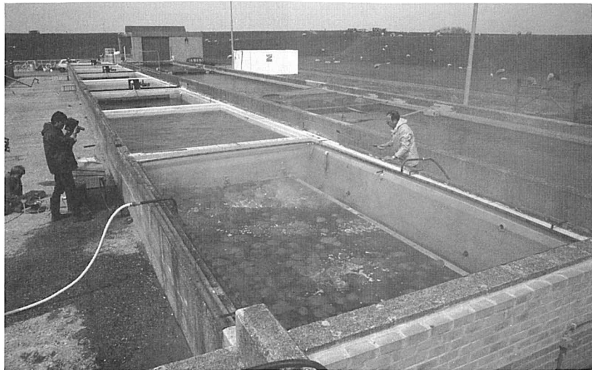
Combatting an oil spill on a Model Tidal Flat by burning.
