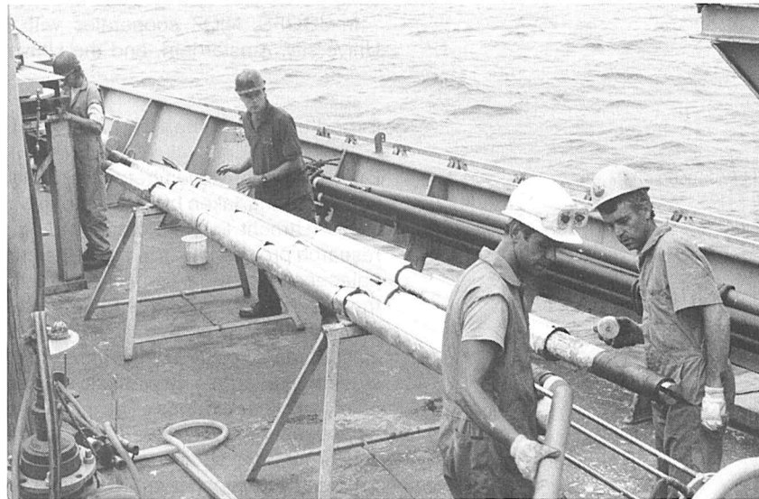
Piston coring. As soon as a core is taken it is thermally insulated on deck with Jacosol pipe insulation, a polyurethane-foam tube which is covered with PVC foil with aluminium coating. The tube protects the cores from heating by the tropical sun until the core is divided into sections and stored or handed to the geochemists.
