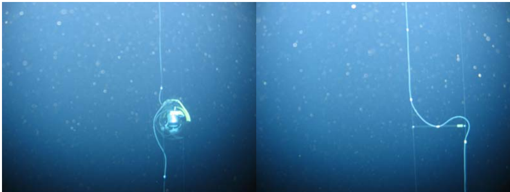
Fig. 10. ROV underwater video stills of upright LOM2-DU. The white line is the VEOC, which switches the barely visible black Dyneema lines every two out of three bars (right), and goes in and out a DOM (left).
