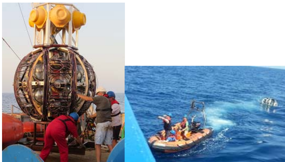
Fig. 4. (left): Fully laden LOM just before deployment. Below the LOM the bottom weight and video camera are partially visible. Above the LOM, its own acoustic release is between six plastic-capped glass spheres. (right): recovering the 'empty' LOM after surfacing.
