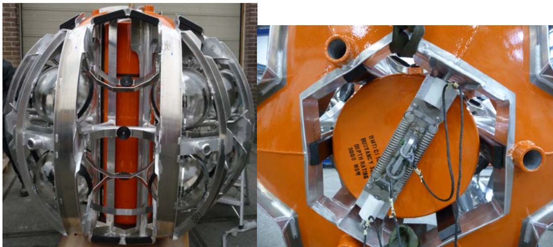
Fig.3. Syntactic foam topbuoy inside the (empty) LOM (left). Top-buoy release mechanical mechanism (right).
