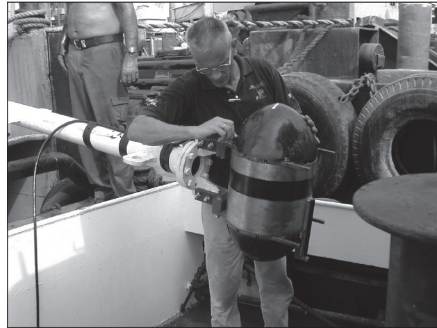
Photo 2: Multibeam transducer being attached at the extremity of a steel pole.
