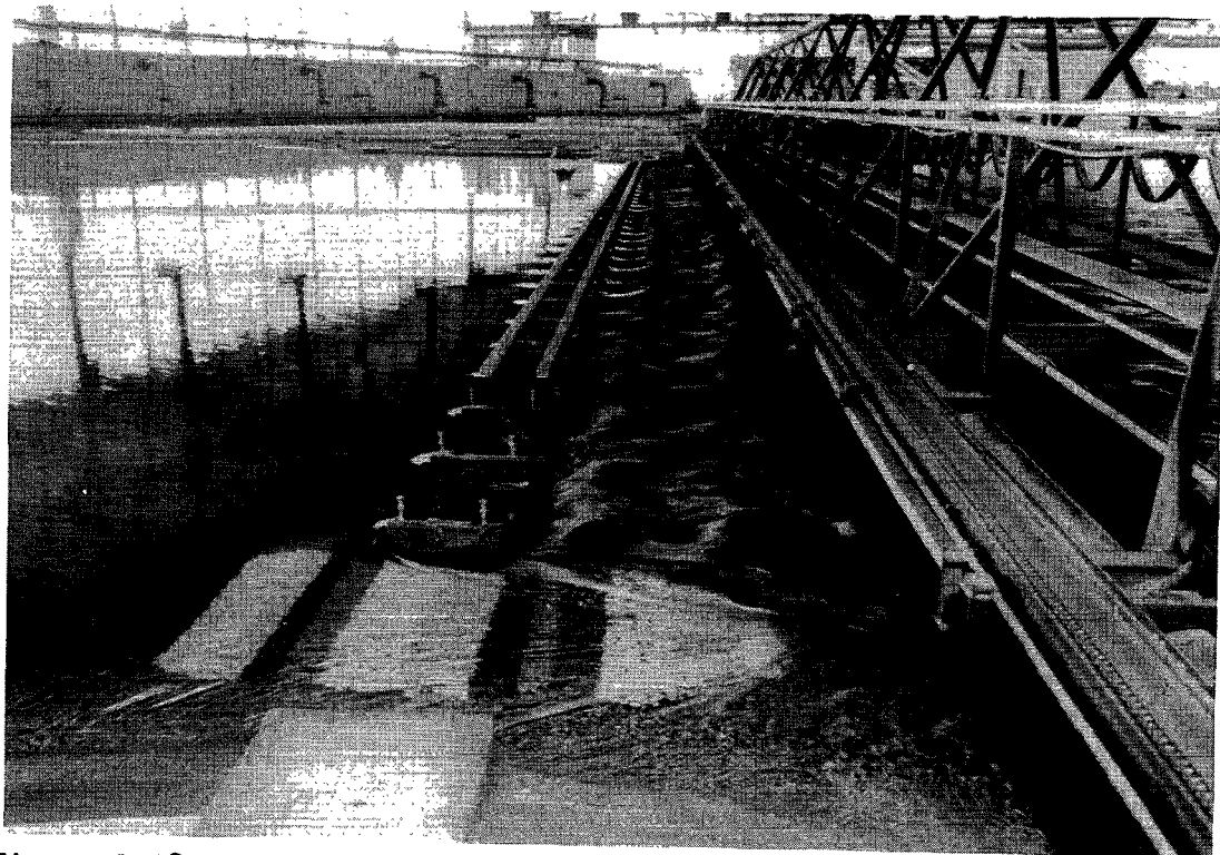
Figure 5.18 Flow pattern at stability test for compartment between first pier and abutment
