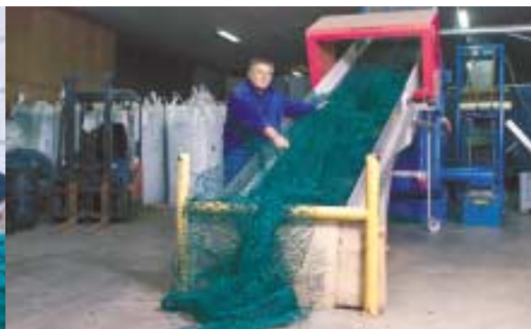
Jens Lundholm Pedersen from Skagen Education Center is in charge of the pilot project to recycle plastic material. The recycling machine takes all plastic marine litter ranging from old netting and buoys to float and fish boxes. Photo: Stig Hedström
