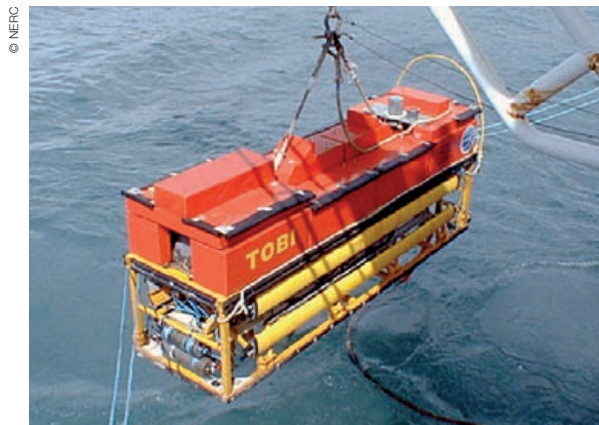
TOBI, a seafloor mapping system
