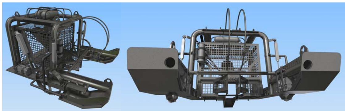
Fig. 1. Artist impression of the Triple-D (side and front view) without the net attached at the back of the cage.
