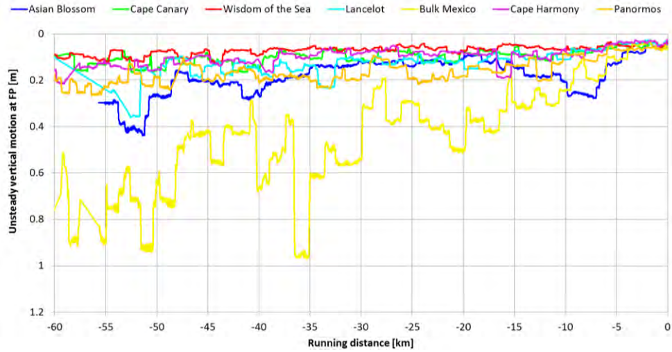
Figure 14: Unsteady vertical motion at bow (envelope) for seven full-scale measurements
