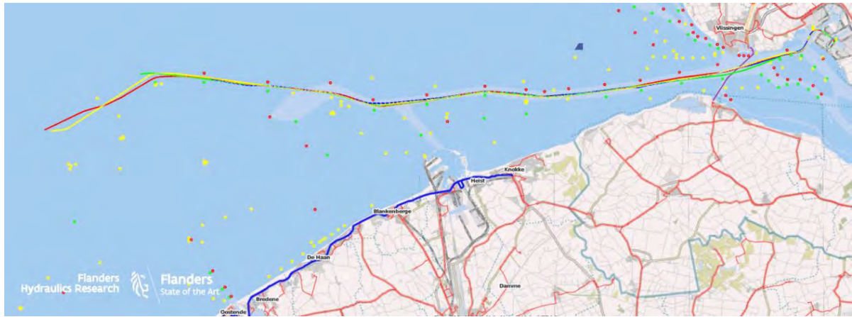
Figure 2: Measured trajectory for 4 bulk carriers sailing inbound to the port of Flushing/Vlissingen (NL)
