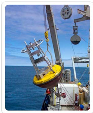
Chilean DART buoy deployed off the coast of northern Chile. Credit: SHOA
