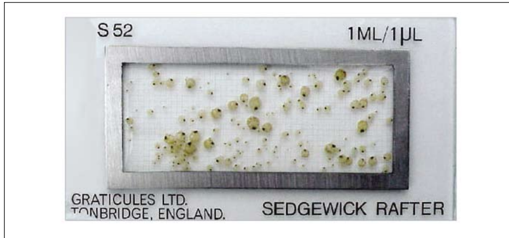
Figure 1.12: Measuring eggs or larvae on a Sedgewick-Rafter cell.
