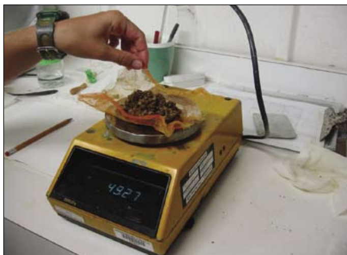
Figure 4.5: Weighing spat on a Sartorius balance ( \pm 0.01 gram).
