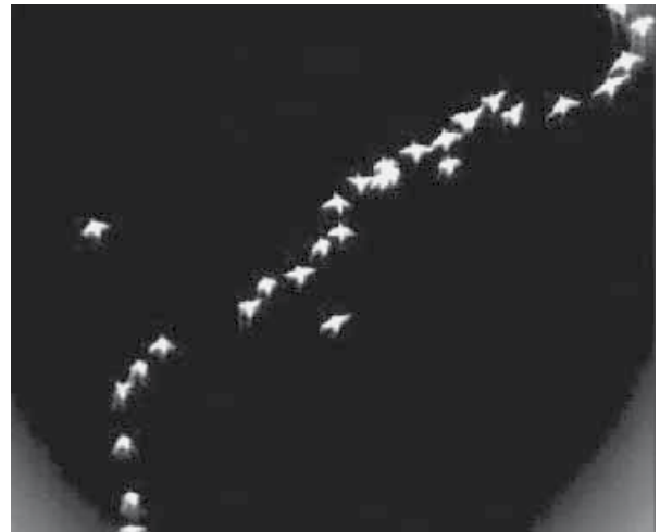
Figure 3. Thermal image recorded by TADS and showing a flock of Common Eiders passing the field of view at a distance of c. 70 meters.
