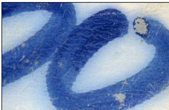
Figures 15 a and b. Permanent Marker OH. Close-up on writing on PE-bag after one year of exposure (left) and on reference sample (right)
