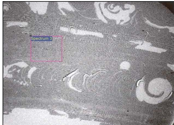
Figures 4 a and b. Retrieved archaeological clear glass sample (left) and SEM image of the clear glass sample (right). The marked area is the weathered layer, the light spiral design is where it has flaked off.
