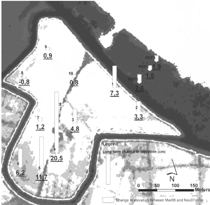
Figure 13 – The change of the sediment surface elevation for the different SET measuring sites after 18 months. The small numbers left-above the white dots are the measuring site labels (cf. Figure 2), the greater underlined numbers are the sediment surface changes in elevation (in cm) after 18 months.
