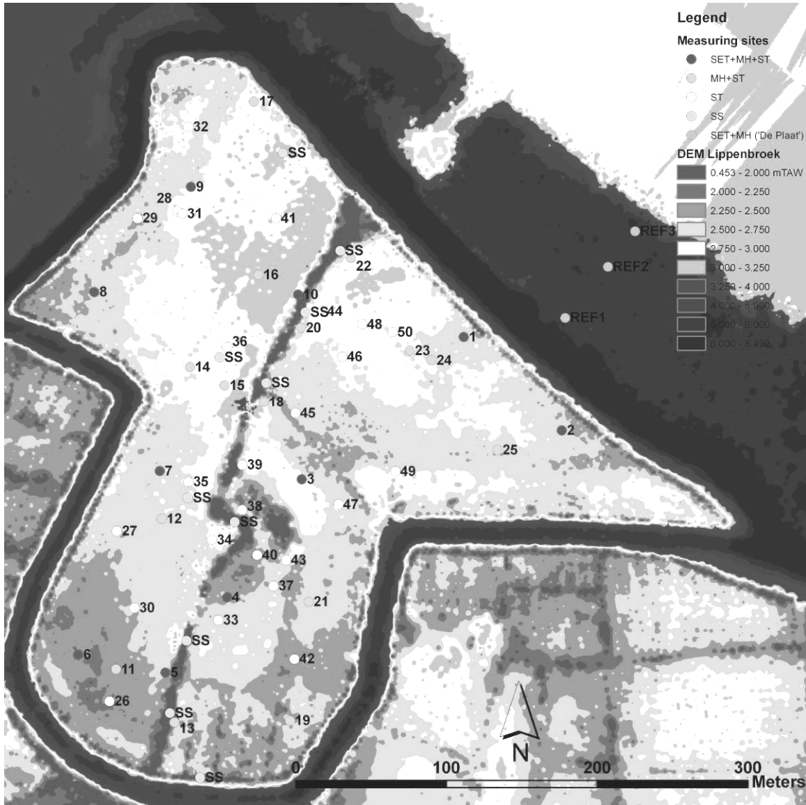
Figure 2 – Measuring sites for short- and long-term sedimentation plotted against a DEM of the Lippenbroek and surrounding area. Dark pink dots represent measuring sites with STs, MHs (marker horizons, explanation below) and SETs (surface elevation tables, explanation below), light blue dots are measuring sites with STs and MHs, white dots represent sites with only ST measurements and the light pink dots are the SS measuring sites. The orange dots are SET and MH measuring sites on the nearby Scheldt marsh 'De Plaat'. SS measuring sites are labeled with "SS", other measuring sites are labeled with numbers ranging from 1 to 50, or with the code "REF" for the marsh 'De Plaat'
