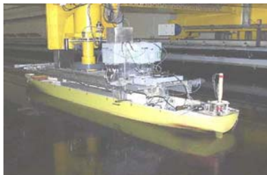
Figure 2. Ship model during captive manoeuvring test.
