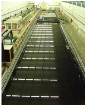
Figure 1. Towing tank for manoeuvres in shallow water.
