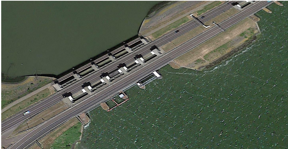
Figure 3.3: Aerial overview of the test site at Den Oever. The first tidal turbines in sluice 2 (from left to right) and the setting of 3 turbines in sluice 4. For this project the turbine in sluice 2 was used.
