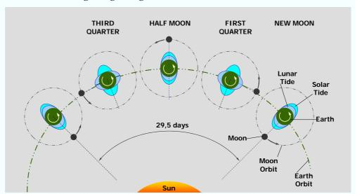
The vertical water movements associated with the rise and fall of the tides are accompanied by roughly horizontal water motions termed *tidal currents*. It has therefore to be distinguished between *tidal range energy*, the potential energy of a tide, and *tidal current energy*, the kinetic energy of the water particles in a tide.
