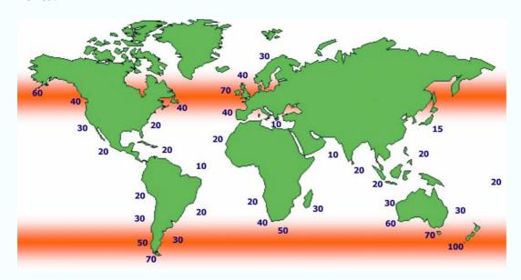
Situated at the end of the long fetch of the Atlantic, the wave climate along the western of Europe is highly coast energetic. Higher wave power levels are found only in the southern parts of South America and in the Antipodes. Resource studies assign for the area of the north-eastern Atlantic (including the North Sea) available wave power resource of about 290 GW and for the Mediterranean 30 GW.
