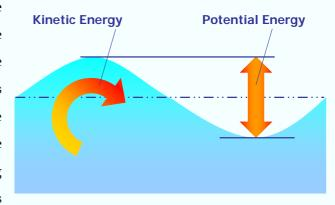
commonly exceeds 40-50 kW per meter width of oncoming wave.
