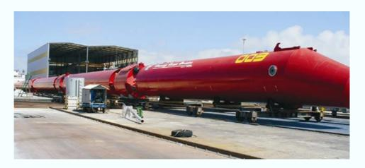
In the period 1998 – 2004 Pelamis has been undergone wave tank and open sea testing at scales ranging from 1/80 to 1/7. In 2004 a 750 kW commercial-scale prototype was installed at the European Marine Energy Centre in Orkney. The prototype is 120m long, 3.5 m in diameter and contains three 250 kW power modules.
