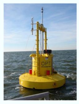
Commencing in 1997, the PowerBuoy has undergone ocean testing in the Atlantic and Pacific Oceans. In June 2004 and October 2005 40 kW units have been deployed off the coast of Oahu, Hawaii, to demonstrate wave power for use at US Navy bases. Another 40 kW demonstration unit was put in operation in October 2005 at Atlantic City, New Jersey.
