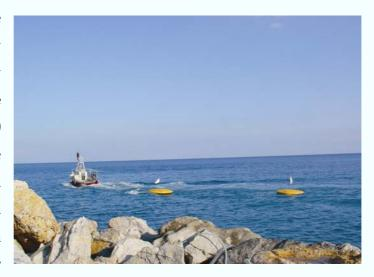
For power production, the pressurized water is supplied to a power take off system on shore, which comprises a patented smoothing accumulator and a hydraulic motor. The motor drives a synchronous generator at  $\sim$ 3000 rpm. In the case of a floater array, several floaters are connected to a common PTO. The electrical power output is estimated to  $\sim$ 2-3 kW per floater at moderate wave power levels ( $\sim$ 10 kW/m).
