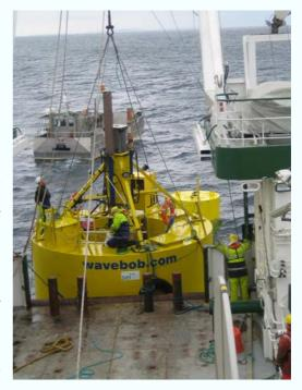
In the past years the concept has been analysed, and the theoretical basis, which comprises frequency and time-domain simulation models, has been verified by independently run tank tests at various scales. A semi-scale (1:4) prototype is currently being tested in Galway Bay in Northern Ireland. One of the aims of these tests is the verification of the time domain modelling approach to explore alternatives, and to test for an optimum device performance.
