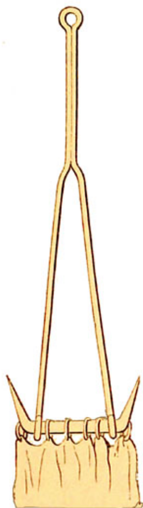
FIG. 49.—The End of the Dredge-frame, showing the mode of attachment of the Bag.
