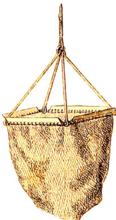
FIG. 44.—Otho Frederick Müller's Dredge. A. D. 1750.
