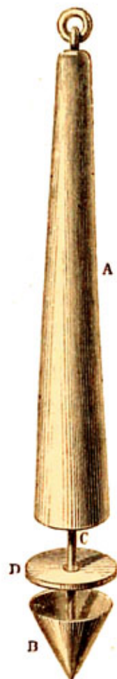
FIG. 37.—The 'Cup lead.'
