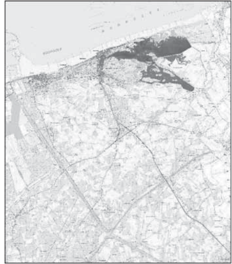
Figure 4b. Flooding caused by a storm with a return period of 4000 years (fine grid with linear elements).
