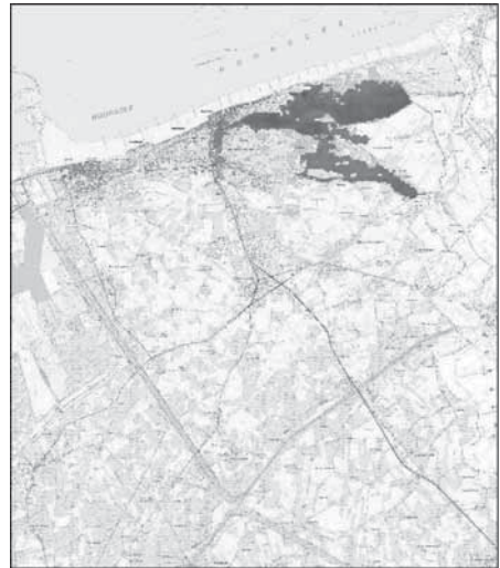
Figure 4d. Flooding caused by a storm with a return period of 4000 years (coarse grid with linear elements).
