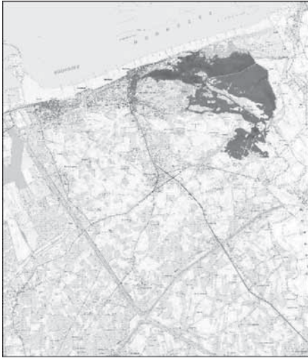
Figure 4a. Flooding caused by a storm with a return period of 4000 years (fine grid).
