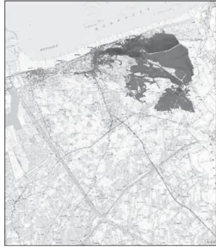
Figure 5b. Flooding caused by a storm with a return period of 10000 years (fine grid with linear elements).
