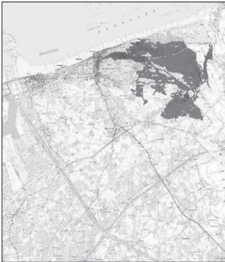
Figure 4c. Flooding caused by a storm with a return period of 4000 years (coarse grid).
