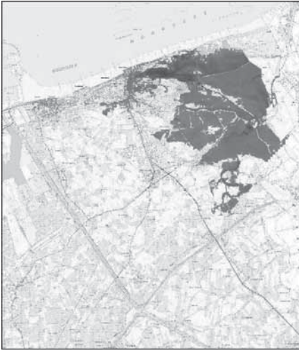
Figure 5a. Flooding caused by a storm with a return period of 10000 years (fine grid).
