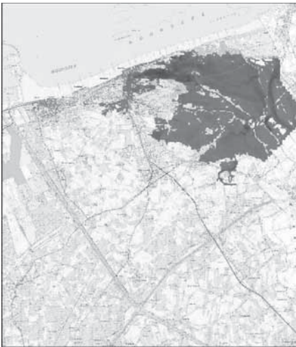
Figure 5c. Flooding caused by a storm with a return period of 10000 years (coarse grid).
