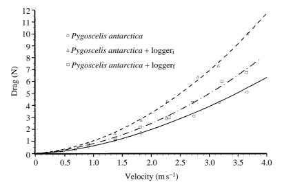
Fig. 4. Drag forces plotted against velocity for undisturbed and instrumented chinstrap penguin models. Logger<sub>i</sub>, initial shape; logger<sub>f</sub>, final shape.
