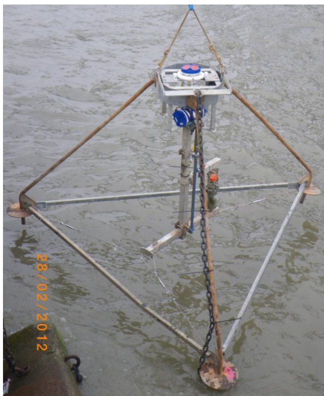
Figure 2-5: A picture of frame CDWup during the deployment of 28/02/2012 including ADCP, RCM-9 and Argus IV. Similar frame is used at location SILL.
