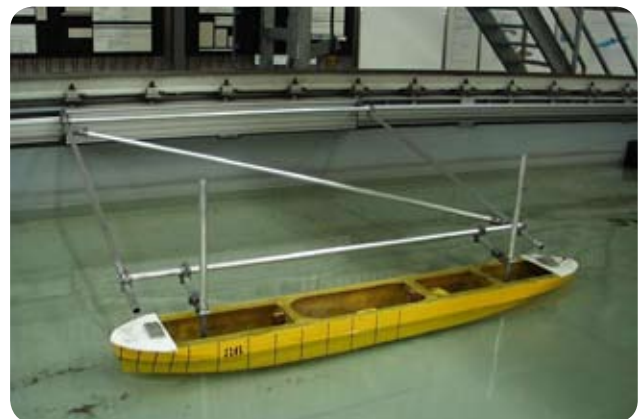
Auxiliary carriage for ship interaction tests
