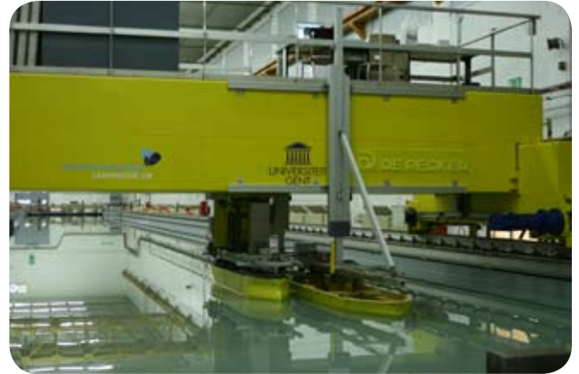
Ship-ship interaction tests: Aframax and VLCC
