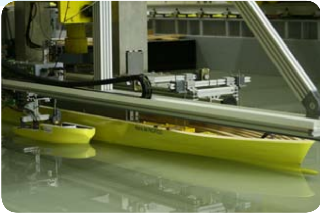
Ship interaction tests: tugboat and Container ship.
