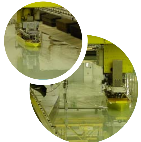
The ship passes along the built-in banks to measure the ship-bank interaction forces.
