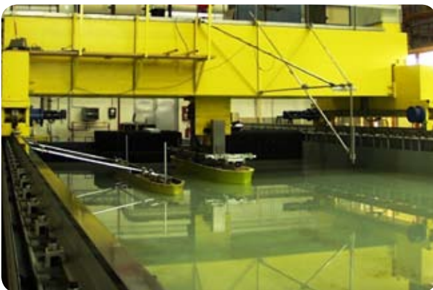
Auxiliary carriage for ship interaction tests
