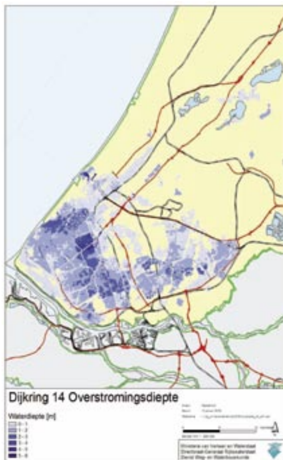
Fig. 4.8 Inundation map showing maximum flood inundation depth caused by a sea flooding event. This example is of Rotterdam in The Netherlands; “Waterdiepte” means “water depth”.
