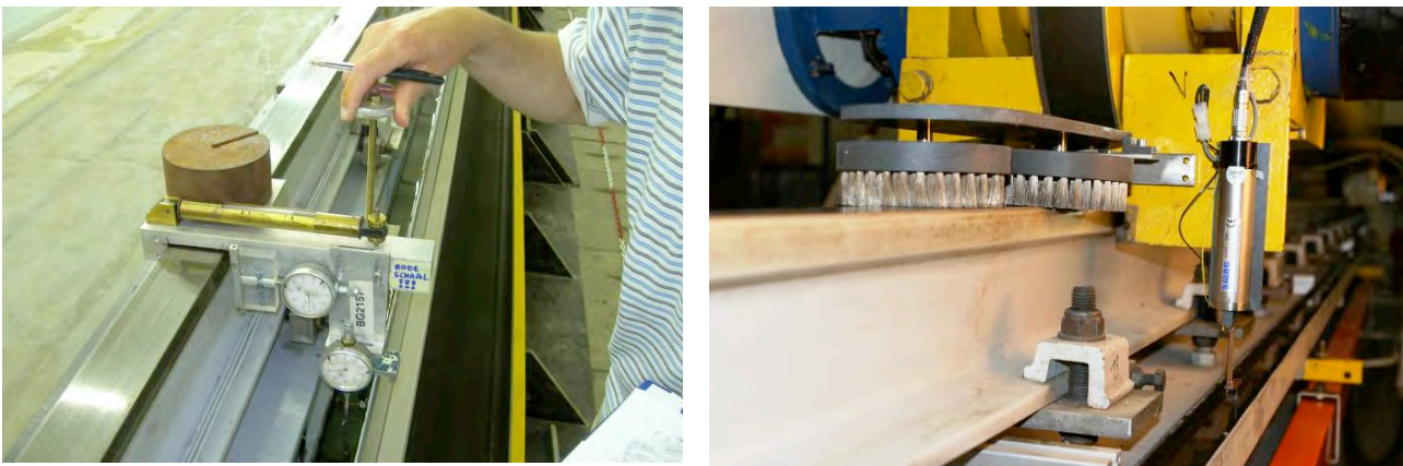
Fig. 15 - Alignment of the rails: manual method (left), electronic method (right)
