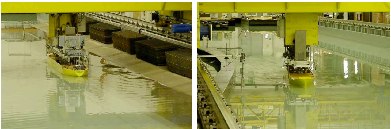
Fig. 11 - Bank effect model tests
