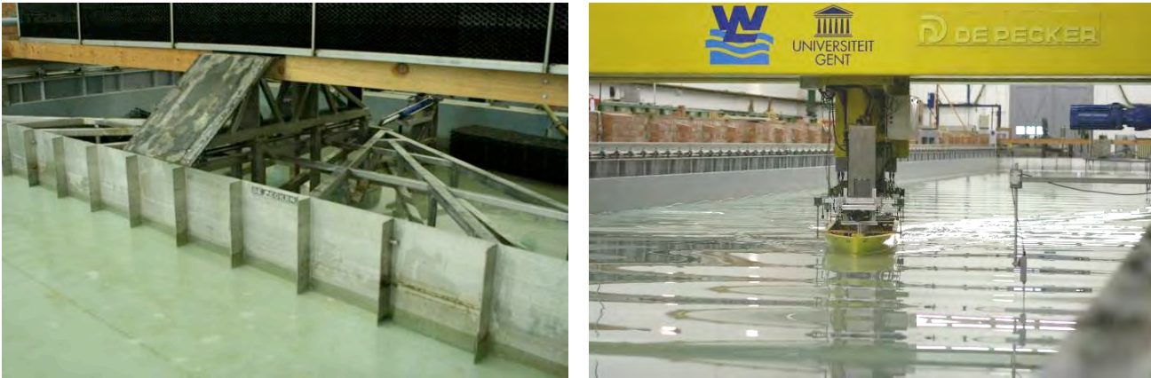
Fig. 8 - Captive sea-keeping tests
