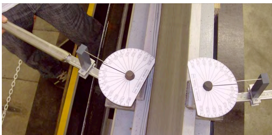
Fig. 16 - Adjustment of the screw bolts with a graduated arc in turn by 0.01 mm
