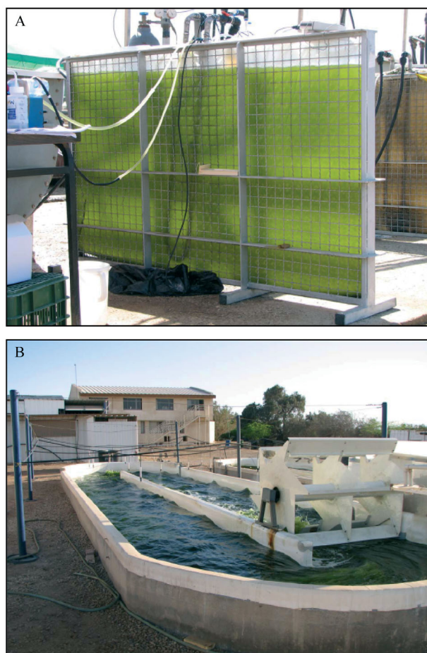
Fig. 1. (A) The flat panel photobioreactor (FPP), constructed of a metal net supporting a flat plastic bag of 5 cm depth. (B) The high rate algal pond (HRAP), constructed of concrete channels with circulation provided by a paddle wheel
