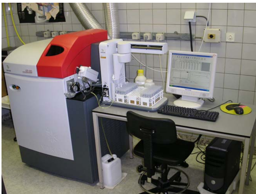
Figure 2.2. Varian Expert 700 quadrupole ICP-MS instrument.
