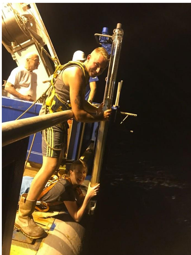
Figure 10.1. Deployment of RAFOS floats on aft deck. Photo credit L. Moerland.
