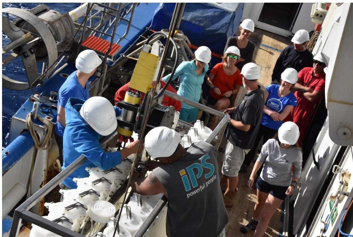
Figure 4.2 Ultraclean CTD is getting ready to be deployed (station 1). Photo credit W. Hooijmans.
