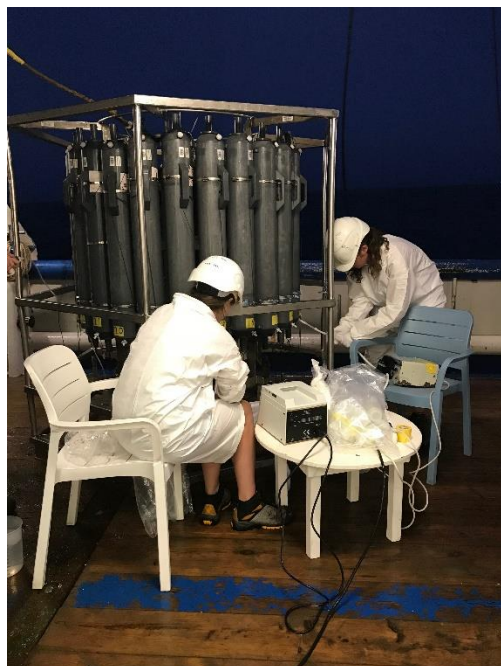
Figure 4.4 Regular CTD Niskin bottles used to collect trace metal samples. Photo credit: Z.Erdem
