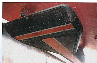
The T-shaped sensor-array mounted in a streamlined gondola under the ship's hull
