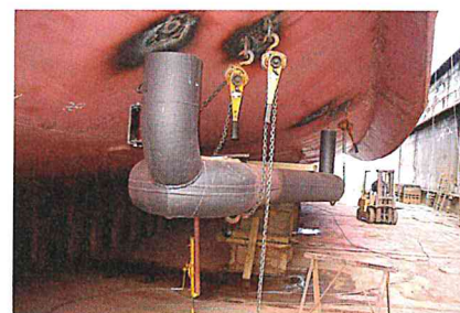
Mounting of the sensor-array under the vessel
