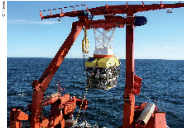
Figure 6. An example of interoperability: deepwater Remotely Operated Vehicle (ROV) Victor owned by Ifremer (France) on board of Research Vessel (RV) Polarstern (Germany)
