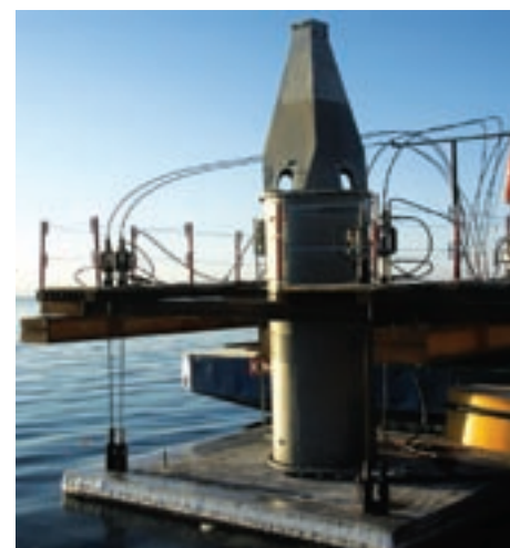
Seabased generator: schematic picture and preparation of the generator for launch off at Lysekil (Courtesy from Uppsala University).
