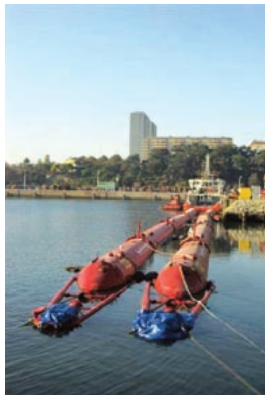
Pelamis machines in Leixões Harbour waiting for installation
