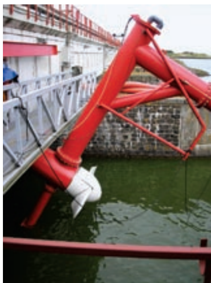
Tocardo turbine by Teamwork Technology, demonstrated at the Afsluitdijk in a sluice gate ( www.tocardo.nl )
