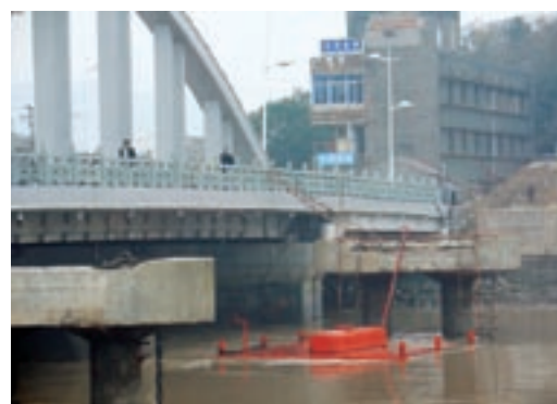
Wanxiang-II 40kW tidal current prototype plant in Zhejiang province
