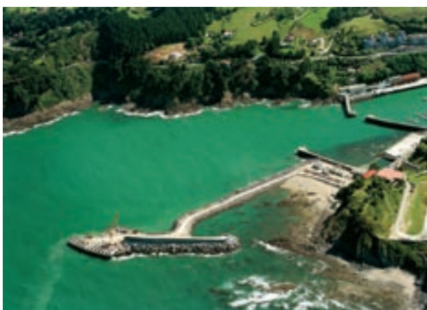
New sea-port of Mutriku under construction with OWC wave energy technology
