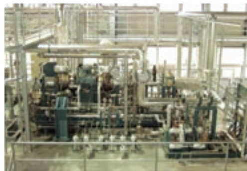
Experimental OTEC plant (30kW) using Ammonia/Water Mixtures as Working Fluid
