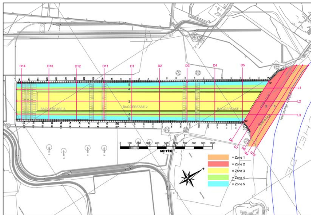
Figure 4-2: Deurganckdok: D and L Sections
