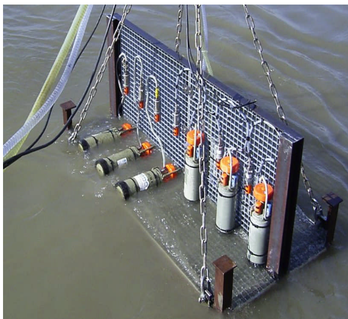
Figure 2-1: Calibration frame with double pump set-up
