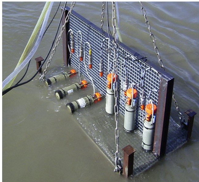
Figure 2-1: Calibration frame with double pump set-up
