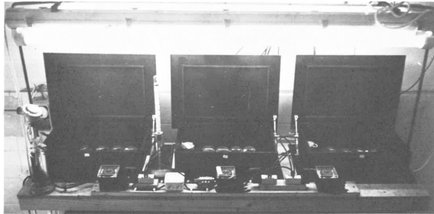
Fig. 1. Culture system used for photobiological experiments. The unit, consisting of three boxes each equipped with automatically opening or shutting cover, is operated in a constant temperature room.
