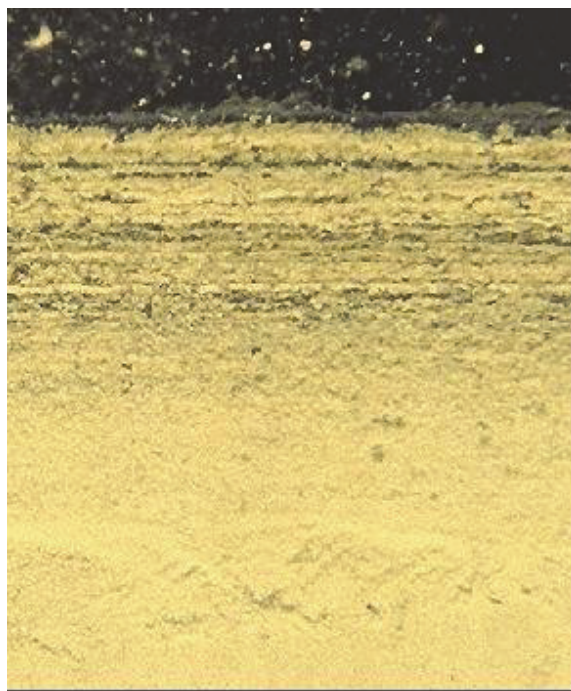
Figure 6. A typical laminated sediment from the open northern part of the Baltic Proper. In situ image taken with a sediment-profile imaging camera from a depth of 125 m. The total length of the image is approximately 10 cm.
