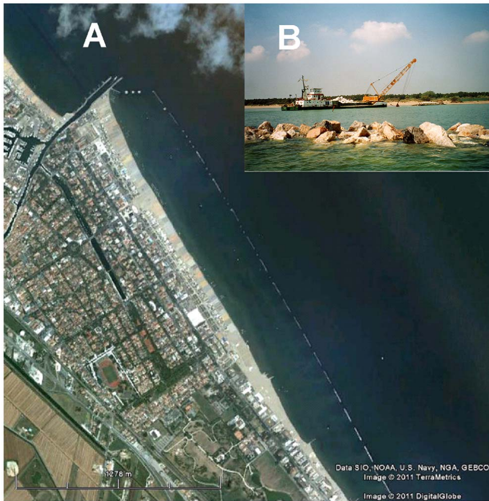
Figure 1. Human-made, coastal defence infrastructures at Cesenatico, along the Italian shores of the north Adriatic sea. A) View of the study area and breakwaters from Google Earth. B) View of a breakwater under maintenance (photo L. Airoidi). doi:10.1371/journal.pone.0022985.g001
