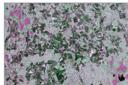
Lääne-Viru County on a false colour composite. SATIKAS uses dense time series of Sentinel-1 radar images as its main data source. Red represents vv-polarization, green vh-polarization, blue vv+vh-polarization.
