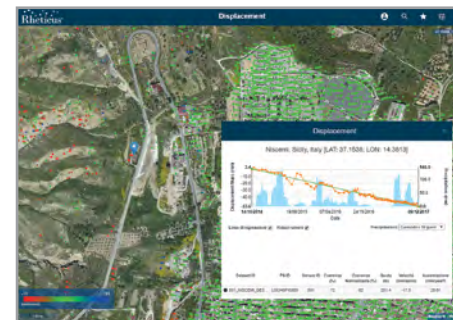
Niscemi, Sicily, Italy. Rheticus® Displacement user interface showing ground movements' velocity acceleration and trends over data retrieved from Sentinel-1.
