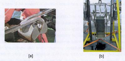
Figure 2.1. The most commonly used sediment sampling devices: (a) Van Veen grabber and (b) box corer
