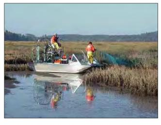
Fig. 7. Airboat with high-pressure spray equipment, Willapa Bay, Washington, USA.
