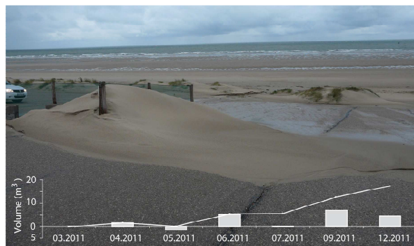
Figure 1 - Evolution of an experimental cross-shaped structure on the windward slope of the dike
