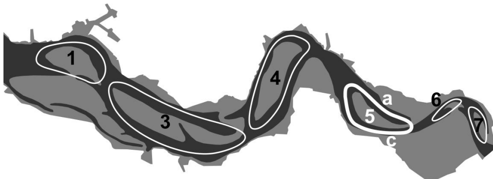
Figure 3 morphological schematization of the Western Scheldt multiple channel system in a chain of cells
