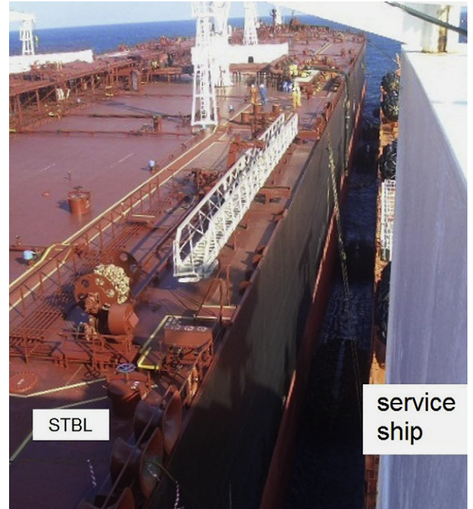
Fig. 7. Picture (courtesy of Yunja Yoo, NTNU) taken from the service ship, the fenders in between both vessels clearly visible.
