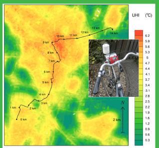
using bicycle-collected data, plus photograph of mobile weather station attached to bicycle. Black line: route
