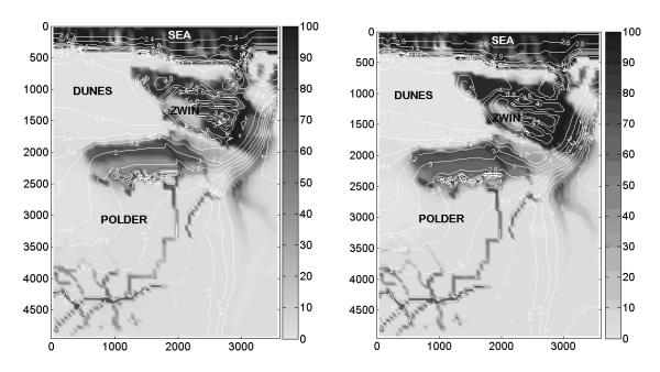
Figure 1. A) Fresh-salt water distribution just below the water table in present situation (white – 100% fresh, black- 100% salt). B) Fresh-salt water distribution just below the water table after 50 years. White contour lines are the freshwater heads in mTAW (=Belgian reference level, 0 mTAW equals 2.36 m below mean sea level).
