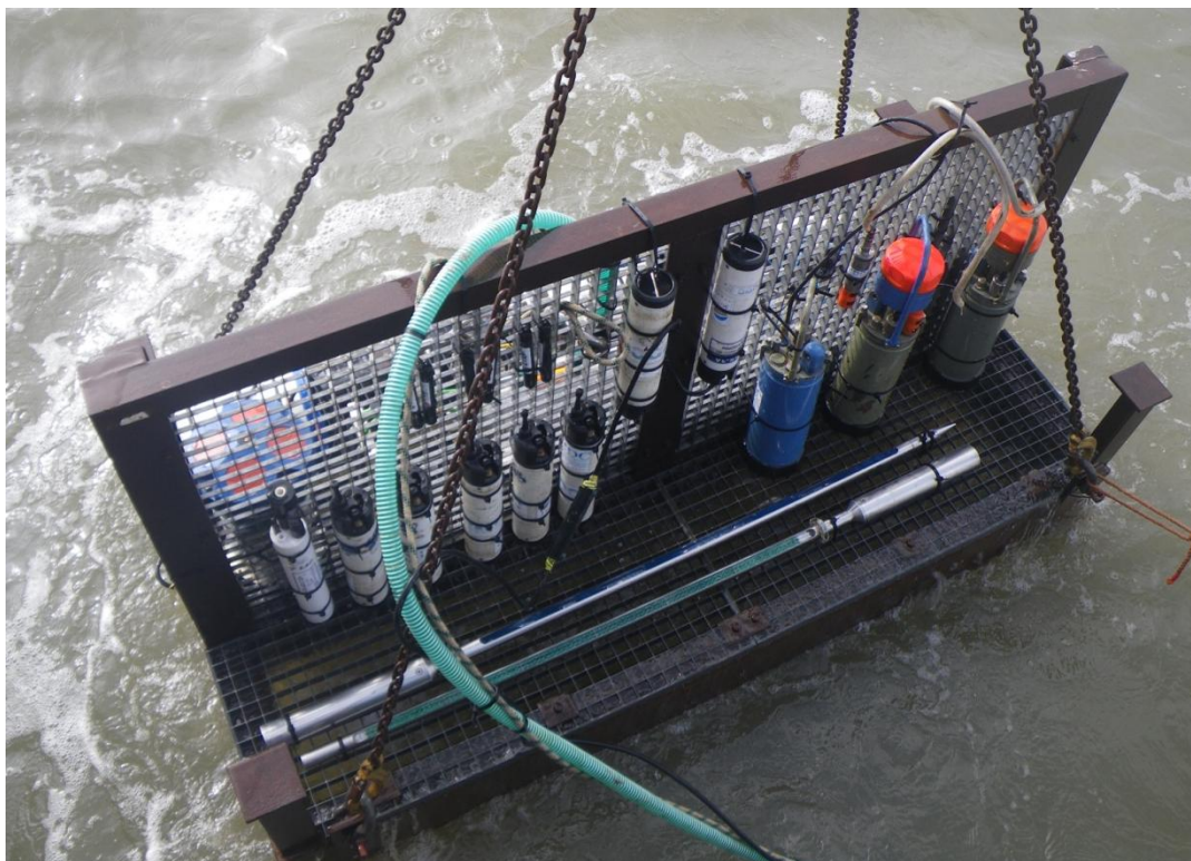
Figure 3-1: Calibration frame with pump set-up
