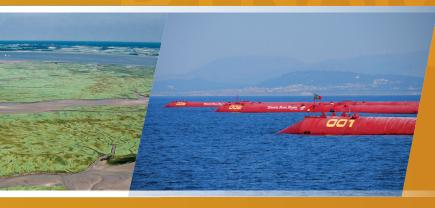
Agucadoura Wave Farm of Pelamis wave energy converters. This mitigation measure is under analysis in the Theseus project.
